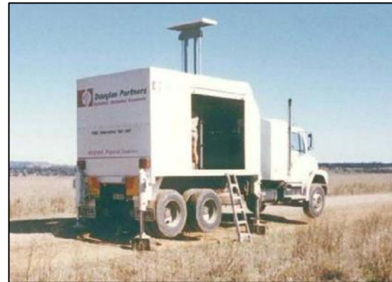
Figure 2: Purpose built CPT rig
